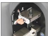
Clamp a key easily with three different clamping positions on the X-Cut's reading vice.
