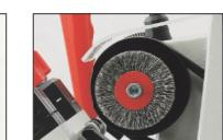
Burrs from cutting to get the brush system of the standard equipment is included.
